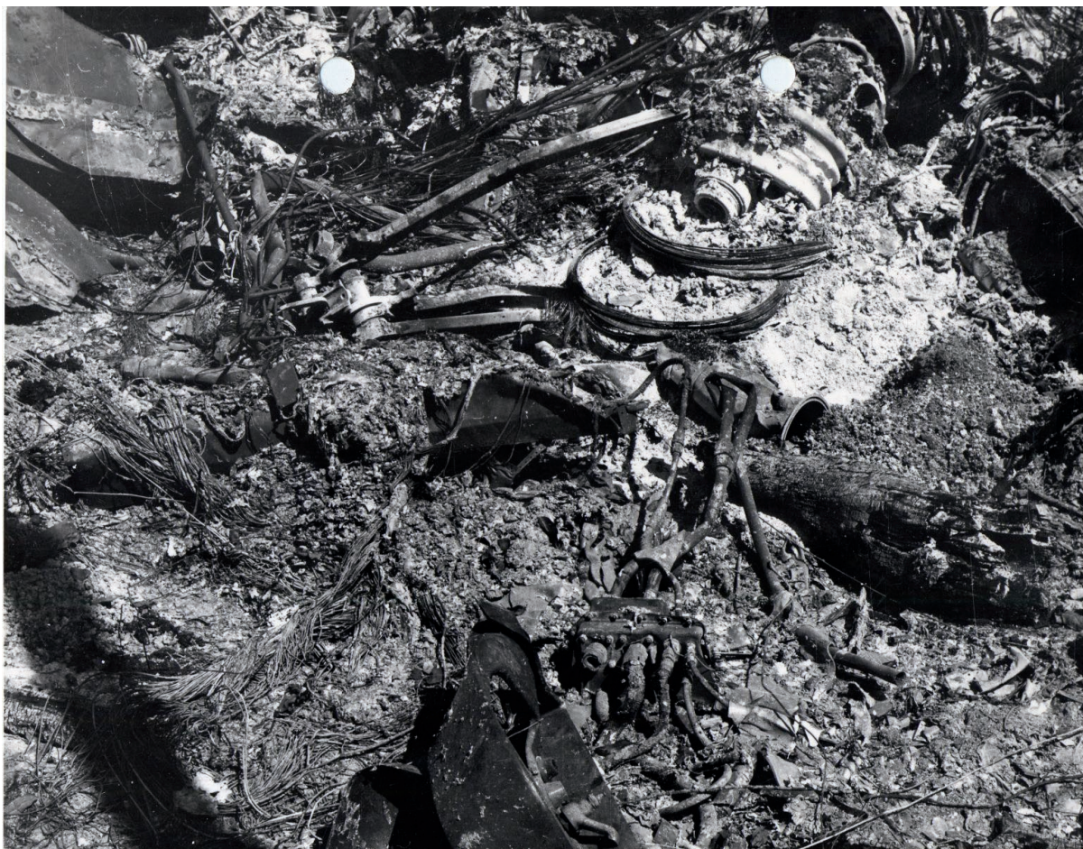
11: Compression-bent retraction links on main landing gear. (# S-0727-0004-01-00018 UN website file.)
